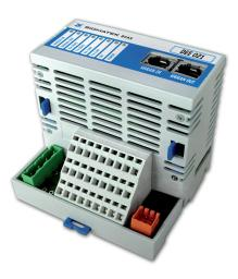
The DEE 021 energy measuring module is used to measure the energy directly on the machine. The voltages from the three input phases (L1, L2 and L3) are measured and up to 12 currents are recorded. The DEE 021 has a real-time Ethernet VARAN as well as a CAN bus interface and can therefore communicate with the automation world perfectly.
