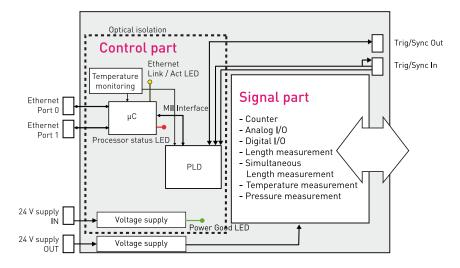
The x-ARTS consist of a signal part and a control part with optical isolation.
